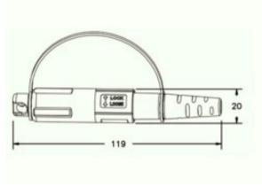
Hardened connector IP67 Protection Operating temperature -40 to 85C
