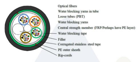
1.2. Identification of fibers and loose tubes
