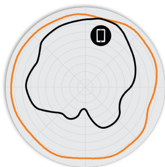
Figure 2. R650 2.4GHz Azimuth Antenna Patterns
