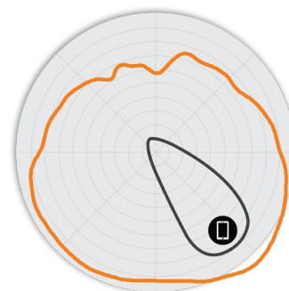
Figure 5. R650 5GHz Elevation Antenna Patterns
