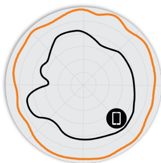
Figure 3. R650 5GHz Azimuth Antenna Patterns
