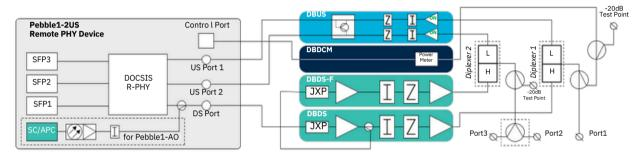
**DBUS** – upstream module / **DBDCM** – control module / **DBDS** – primary downstream amplification module / **DBDS-F** – secondary downstream amplification module / **DBTM** – termination module
