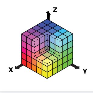
Digitally, this can be broken down into a 3d coordinate space, with red, green, and blue on separate axes and having a range of 0 to 255 (one byte).
