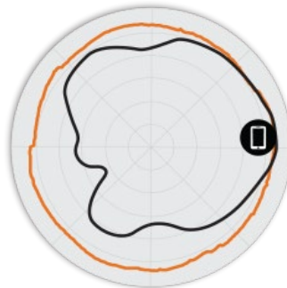
Figure 3. 5GHz Azimuth Antenna Patterns
