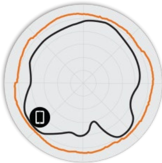
Figure 2. 2.4GHz Azimuth Antenna Patterns
