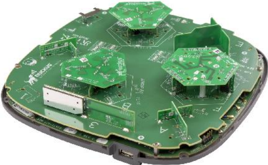
RUCKUS BeamFlex® Smart Adaptive Antenna
