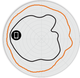
Figure 5. R770 2.4GHz Elevation Antenna Patterns
