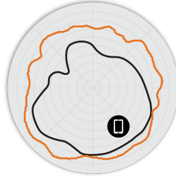
Figure 6. R770 5GHz Elevation Antenna Patterns
